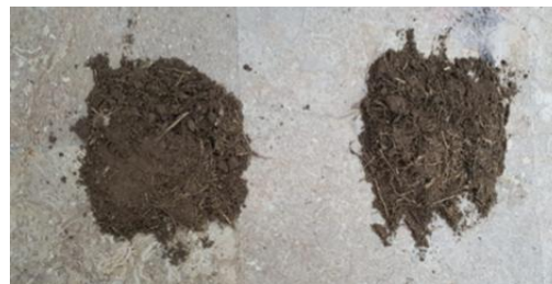
Figure 6 Decomposition of Bagasse Plates Under Soil Conditions Over Consecutive Days
