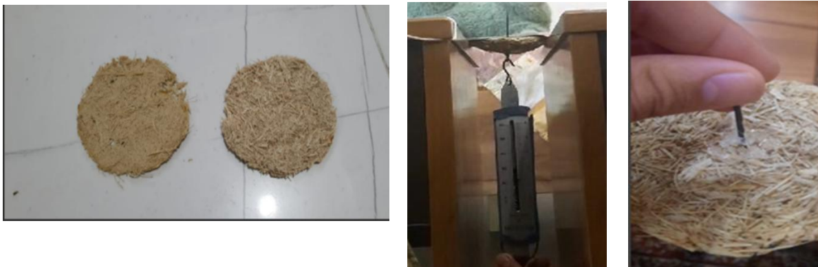
Figure 3 Bagasse plates produced simply baked and boiled water
