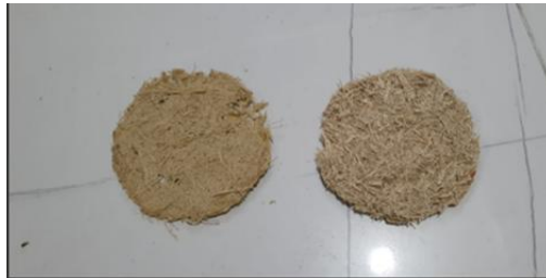
Figure 5 Comparison of bagasse plate samples after immersion in water for 5 minutes.
